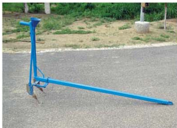
Fig. 43: Two furrow seed drill developed for donkeys
