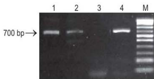
Fig. 73: PCR amplification of fljP gene of B. mallei for diagnosis of glanders Lane 1: Sample 2645, Lane2: Sample 2651, Lane 3: Negative control, Lane 4: Positive control, Lane M: 100 bp DNA ladder
